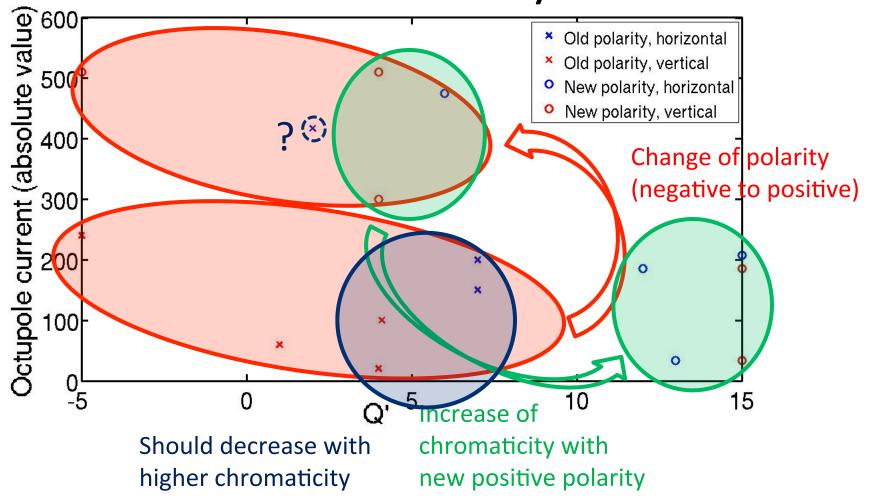
Note: beam and machine parameters are sometimes slightly different between these measurements.
