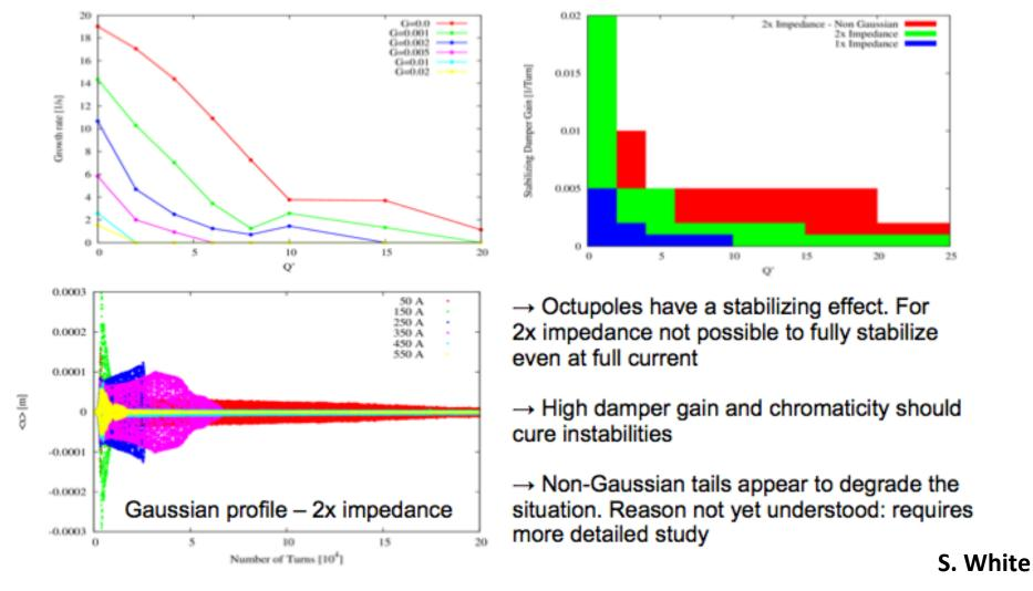
To stabilize LR modes we need very high damper gain and octupoles should be effective but with very high strenght
