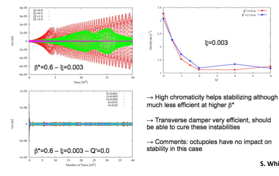
High Chroma and Transverse Damper can damp the coupling of a BB pi mode and impedance but octupoles are not effective
