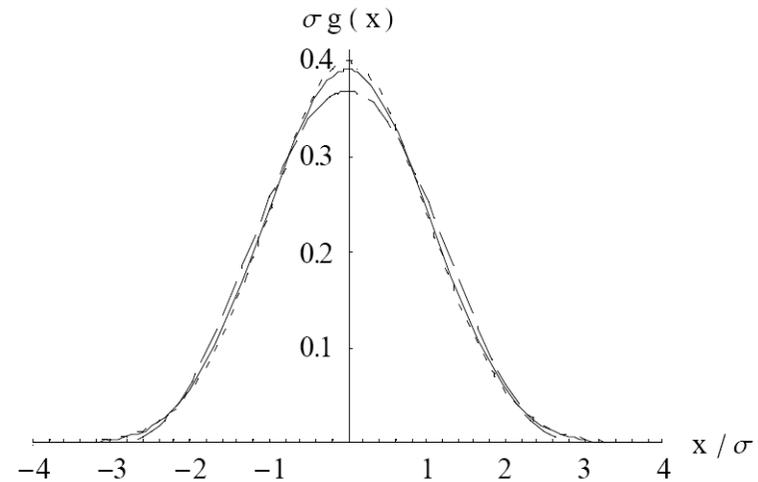
Figure 1: Transverse beam profile for the 15<sup>th</sup> order distribution (full curve), the quasi-parabolic distribution (dashed curve) and the Gaussian distribution (dotted curve).
