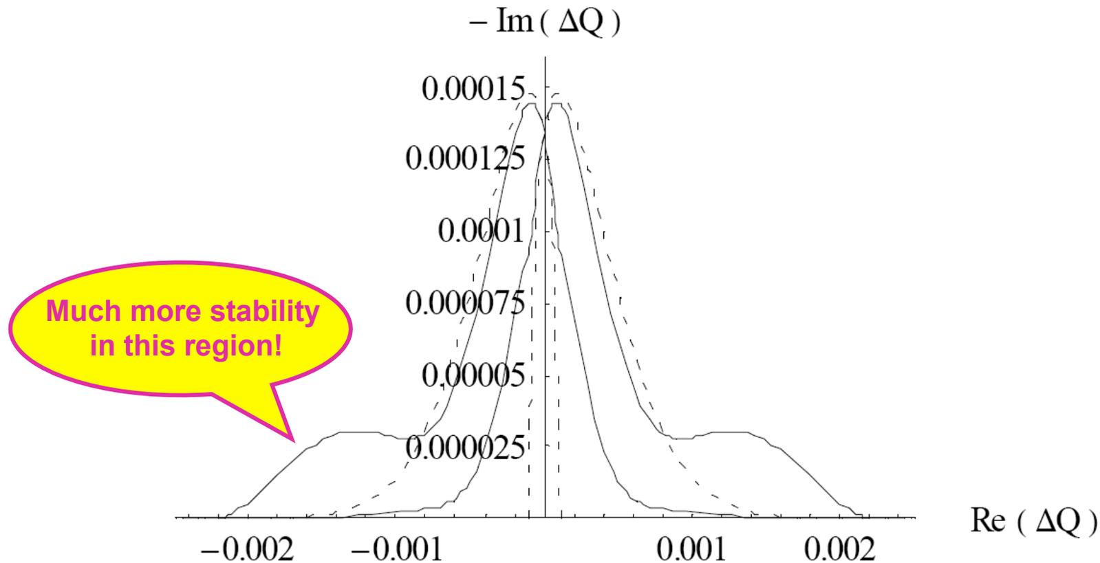
Figure 7: Stability diagrams (positive and negative detunings  $a_0$ ) for the LHC at top energy (7 TeV) with maximum available octupole strength, for the case  $n = 16$  and  $p = 2$  (full curve) and the Gaussian distribution (dotted curve).
