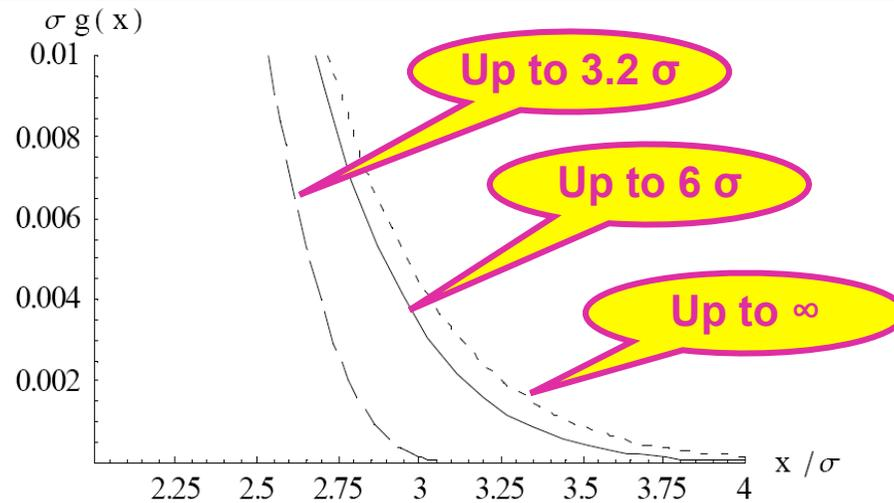
Figure 2: Zoom of the tails of the transverse beam profiles for the 15<sup>th</sup> order distribution (full curve), the quasi-parabolic distribution (dashed curve) and the Gaussian distribution (dotted curve).
