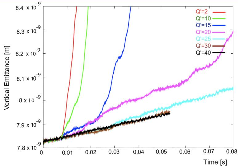
Figure 7.11. Vertical emittance growth for different chromaticities, for LHC at injection,  $\rho_e = 6 \times 10^{11} \text{ m}^{-3}$
