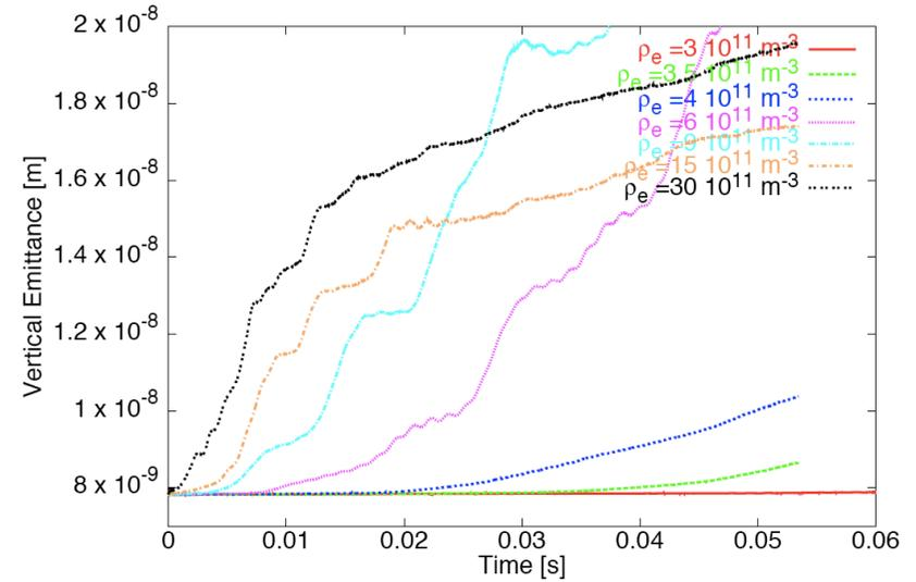
Figure 7.8. Vertical emittance as a function of time for different values of electron cloud density, and  $Q' = 2$  (for LHC at injection).
