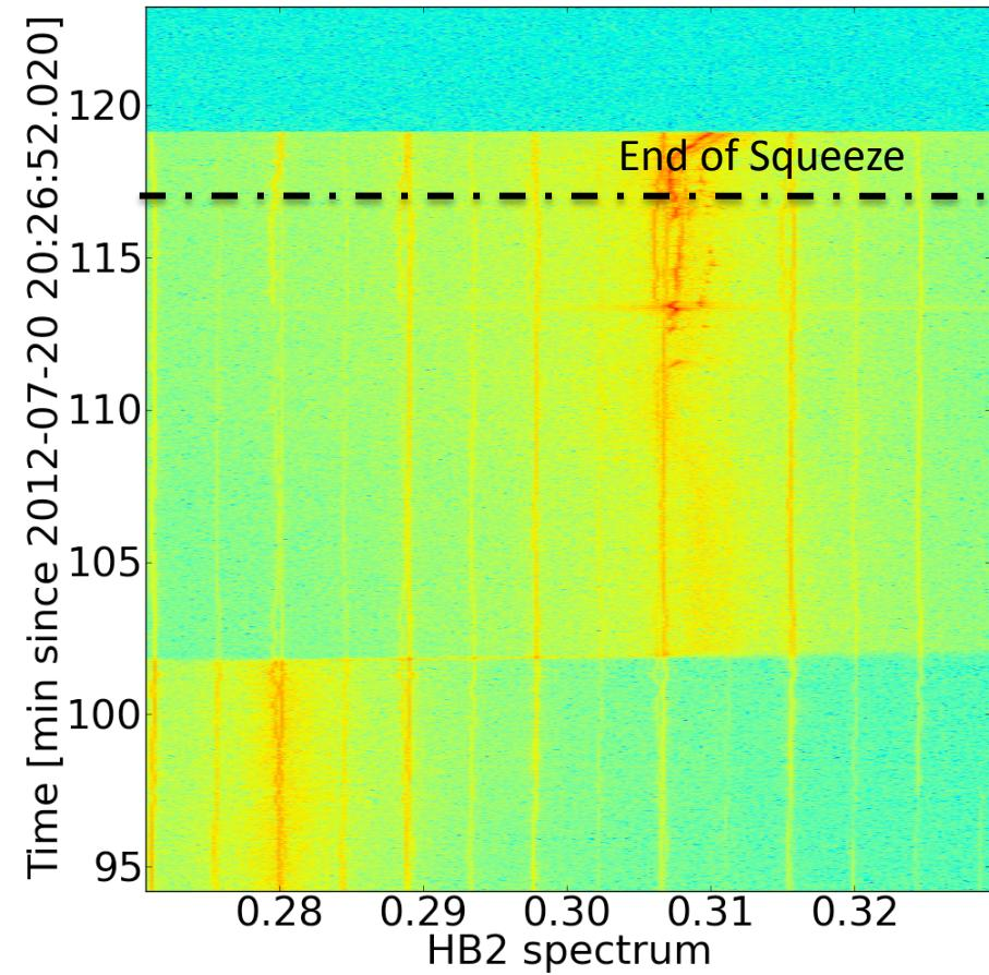
Typical instability **2-3 frequencies** develops before adjust and/or during adjust and propagates for several minutes
