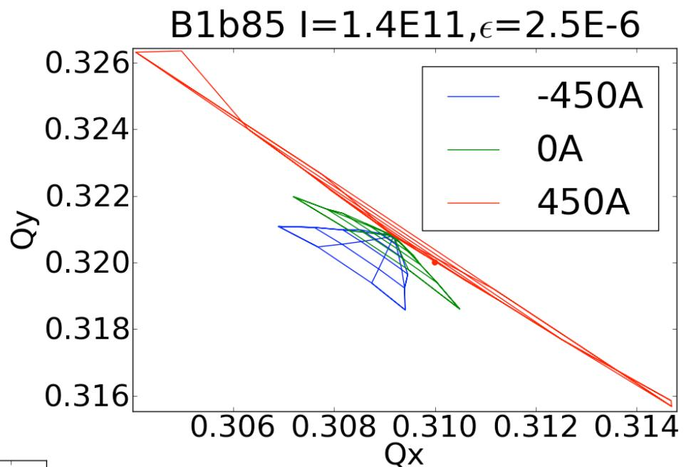
To provide **Landau damping** one need tune spread (BB + Octupoles) and particles at those frequency (assuming Gaussian distribution one has to look at  $3\sigma$  amplitude footprints)
