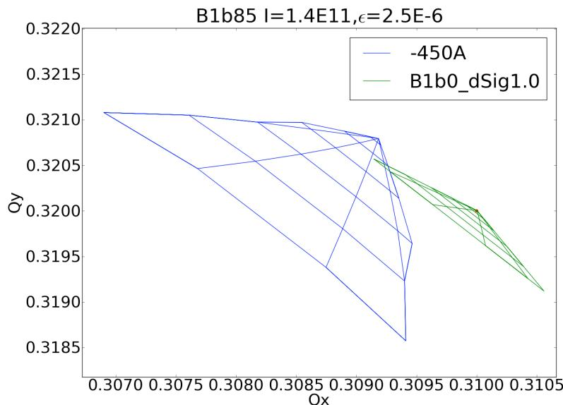
Landau damping provided by -450 A Octupoles + BB compared to what needed on single beam (-100 A )
