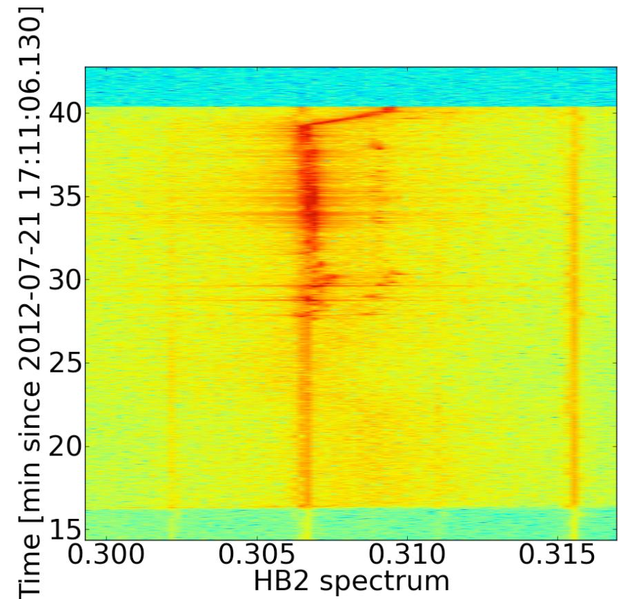
Typical instability **2 frequencies** develop during squeeze and propagates for several minutes
