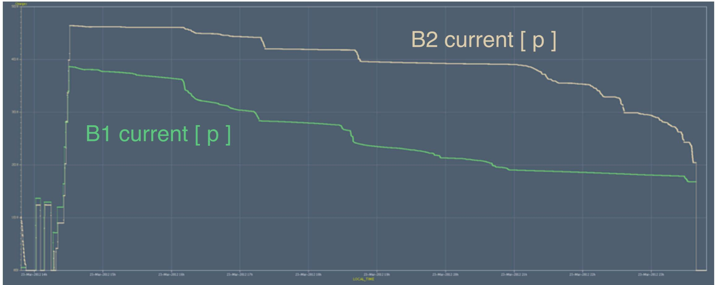
*Injected 7-8 “small” probe bunches of  $\sim 5 \times 10^9$  protons, emittance > 3-4 microns*
