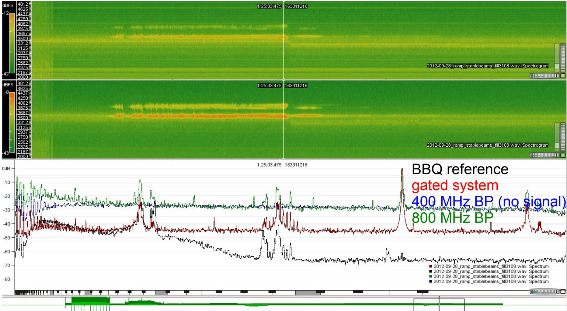
Q-amplitude-to- $f_{rev}$  ratio larger at 800 MHz than <400 MHz  $\rightarrow$  intra-bunch motion
